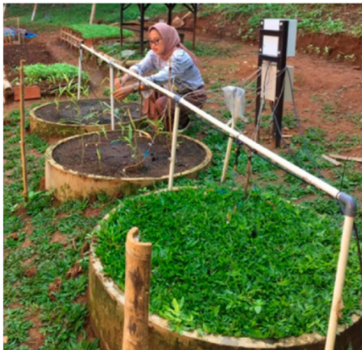
Fig. 1 The lysimeter system used
